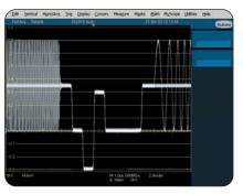
Video Design. Illustration of triggering on an analog HDTV tri-level sync signal and examining horizontal blanking interval.
