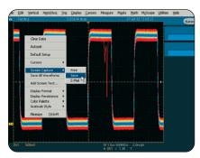
Elusive Glitch. Fast waveform capture rate, enabled by Tektronix proprietary DPX acquisition technology, maximizes the probability of capturing elusive glitches and other infrequent events.
